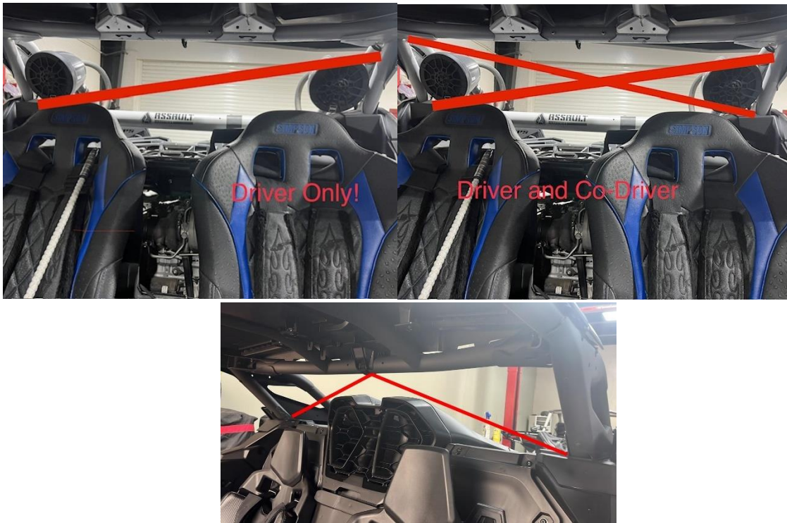
Pic 17.1 Examples of main roll bar brace for both driver and driver/co-driver configuration.
